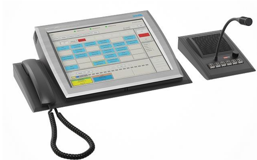
Figure 2: MPD with handset and speaker box with goose neck microphone
