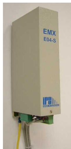
In metallic housing for indoor installation to DIN-rail.
